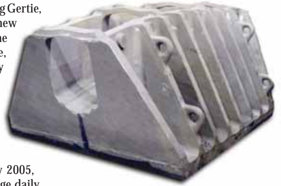
SADDLE UP The 20-ton splay saddle, used on the new Tacoma Narrows bridge, was produced using a nickel-chromium-molybdenum steel alloy.
